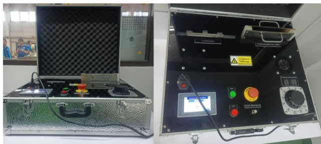
Figure 1. A portable prototype integrating a pulsed electric field (PEF) and ultrasonic system.
